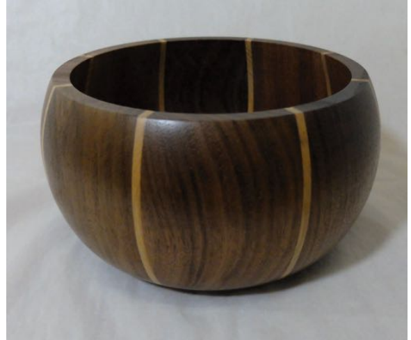
Lionel Hart has made this segmented bowl from Blackwood and Oregon. The finish is Nitrocellulose Lacquer.
