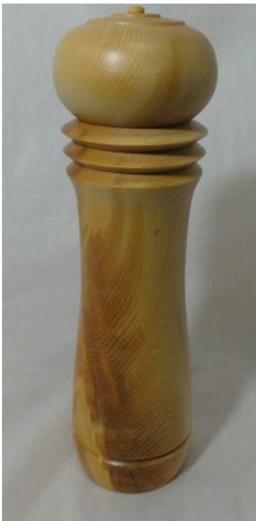
Lionel has also made this pepper grinder from Huon Pine. It is also finished with Nitrocellulose Lacquer.
