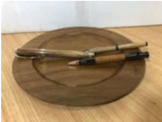
Ian has made this plate from Iroko and finished it with Shellawax. The slimline pen is recycled rain forest timber and finished with CA glue. The bolt action pen is New Guinea Rosewood. The Graduate Fountain pen is Melaleuca.
