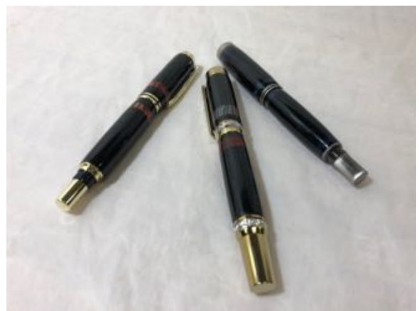
These pens have been made from Indian Ebony. All pens have been finished with CA.
