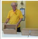
Alan presented this box and advised "This box holds the third Club's Gifkin jig. It was made with 15 mm finger joints using the Club's new 15 mm finger jointer kit. It was made from some of the Club's maple timber planks thicknessed to 16 mm, using some brass hinges and handles from the
