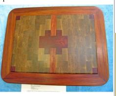
centre is assembled around the Rosewood centre. Around the raised centre panel is Rosewood edging mitred assembled using dominos, including in the mitres."
