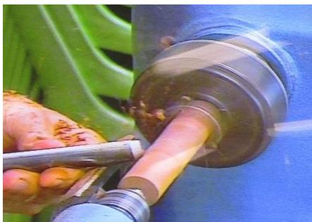
Using a 16mm Forstner drill in a Jacobs Chuck Brian removed the centre section of waste from the end of the blank. He used the standard jeweller’s guide to ring sizes to determine the internal diameter and added the planned ring thickness to determine the outer diameter. Brian turned the tip of the blank to the appropriate diameter and reduced the waste
