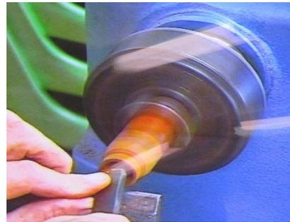
The next stage involved sanding, first with sandpaper – 240g, 320g, 400g and 1200g; followed by micro mesh – 1500g, 1800g, 2400g, 3200g, 3600, 4000g, 6000g, 8000g, 12000g, and 20000g. These involved short, gentle touches. Brian then applied a dot of Shellwax using his finger and a polishing rag.
