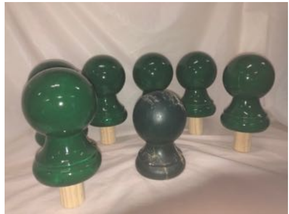
No, not lollipops. Lionel Hart has turned these fence posts for his replacement fence. They are treated Pine finished with paint.
