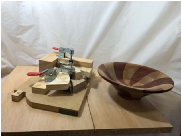
Lionel has shown his segmented bowls recently. Today is showed uo the jig he made to cut the segements accurately on the bandsaw.
