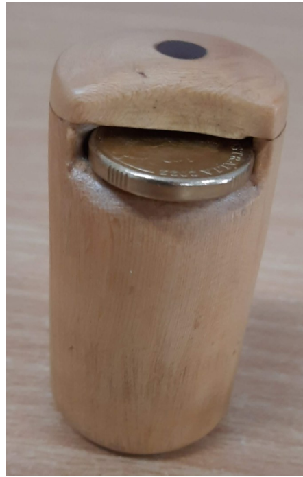
Above: This is spring loaded $2 coin holder made by Brian Johnson. Easy enough to put in a pocket, it takes eight $2 coins.
