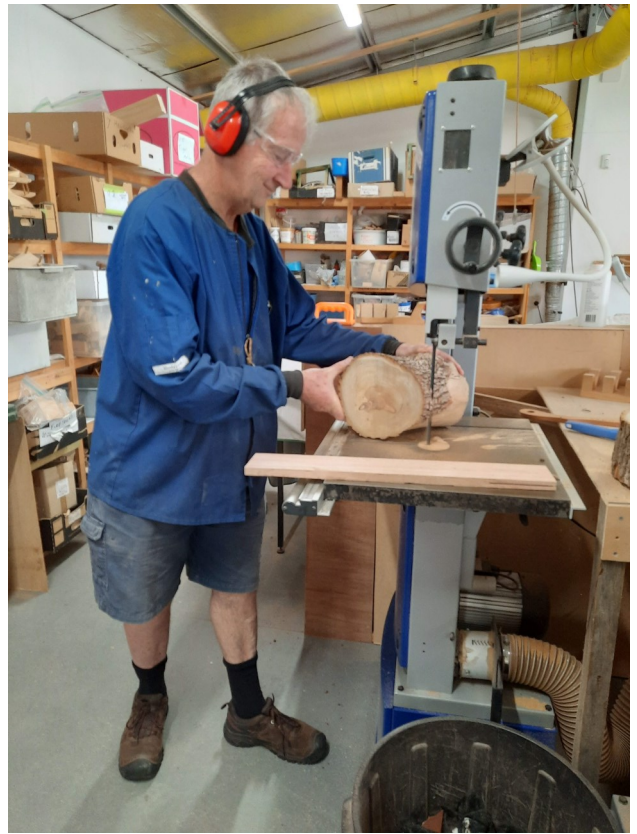
Above: Lex shaping a piece of Camphor Laurel in preparation for turning.
