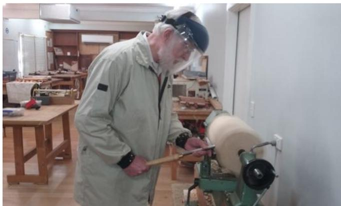
The other photo is of a 200 x 200 x 330 mm glued up pine block being turned into a cylinder. This will form the boiler section of a toddler's ride on steam engine currently being constructed in Wes's Workshop.
