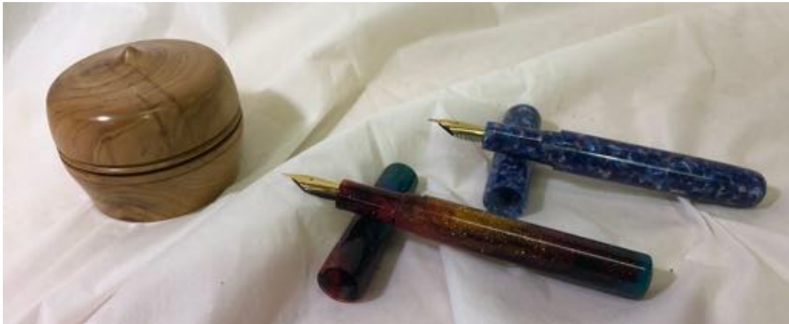
Ian Beckett has made the box from Cyprus and finished it with Shellawax. The 2 resin fountain pens are kitless pens – Ian has turned the threads in these pens.
