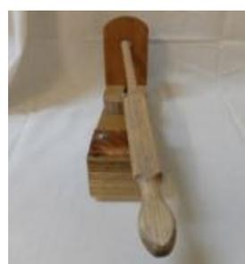
A knife sharpener by Gordon. There is a slip stone on the other side of the handle. The back view shows how the handle can pivot while using the sharpener. The finish is polyurethane lacquer.
