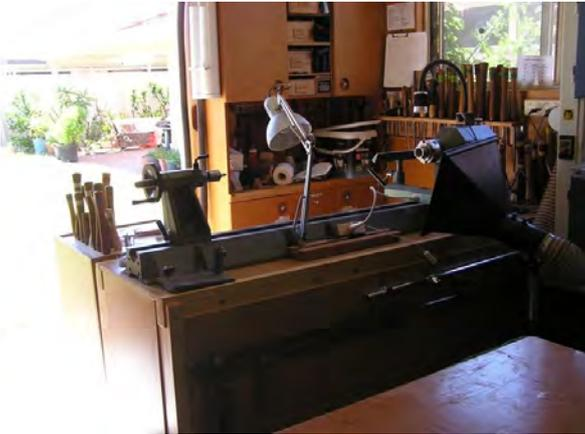
*Plate 2: Looking towards the door, showing the cupboard/workbench on the eastern wall. The structure of the lathe stand is evident. Note also the mobile tool trolley at the right hand end of the lathe.*
