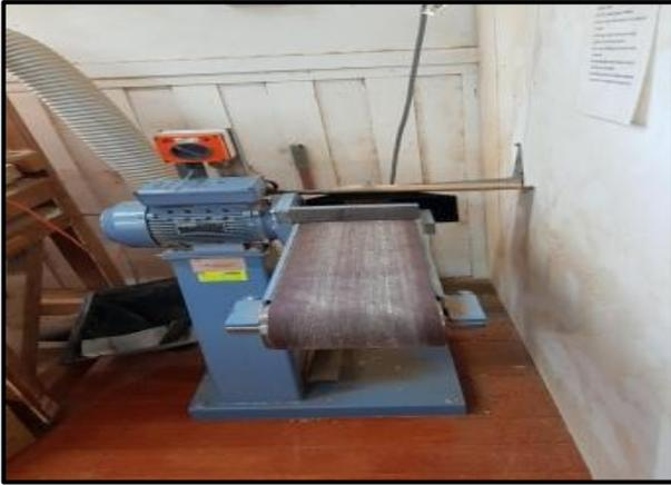
Henry has been trying to improve the dust extraction on the finisher and today completed fitting a dust chute made for the job. The additional installation of a flap to help break the flow going over the finished made a noticeable difference to the dust collected.
