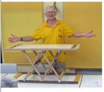
Maurice presented this scissor lift and advised "My scissor lift device. I was looking for a means of raising the height of a small, somewhat weighty, Ryobi bandsaw to use at a comfortable height instead of it being placed on my home workbench taking up too much bench space as well as being too high for comfortable use. I have a small workbench and
