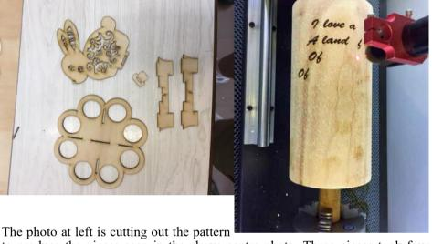
to produce the pieces seen in the above centre photo. These pieces took four minutes to cut out of 2.9mm plywood. The photo at right is the first try at engraving on a round pieces of wood using the rotating device. The bottom photo shows some of the happy members looking at the new toy working.
