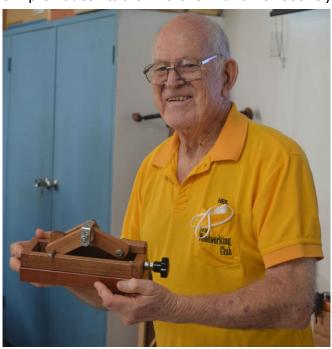
donated to the club. The procedure after changing a router bit is to unclamp the router, raise it a little higher than you need and clamp the router. Place the lifter firmly under the router, unclamp and lower the 'lifter' to the required height of the router bit, clamp the router and start work.
