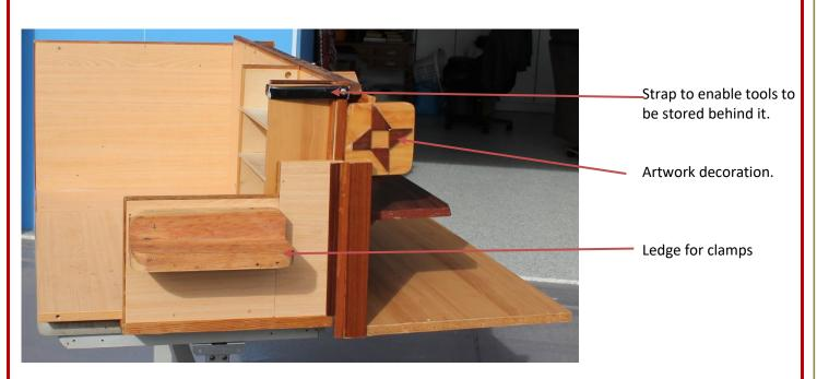
Above is a side view of bench showing a bit of artwork, a ledge for clamps, and a place for some tool storage.
