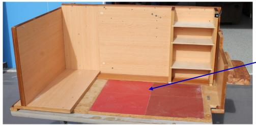
Removal of the slide out bench top reveals sand paper glued to bench. Note the two different grits.
