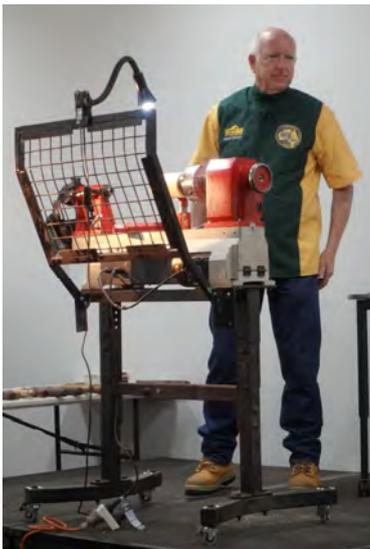
First up was Denis Tapley whose demonstration was turning spheres then embellishing them. Naturally, there are different ways of turning a sphere and Denis made it look quite easy to do without a jig to help. The spheres produced were mostly about the size of a cricket ball.
