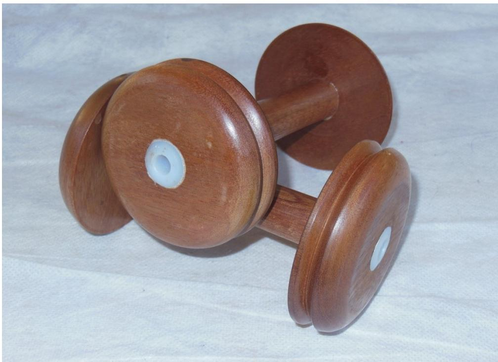
The above items are bobbins for an electric spinning wheel. One of the spinners purchased the spinning unit and requested the extra bobbins to be made. I have fitted a nylon section each end as a better wear surface on the metal shaft, the original ones have a brass section for the wear surface.
