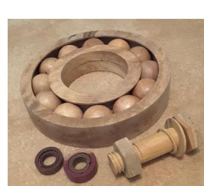
Another challenge is to make a simple ball bearing, just being 1mm out with either the balls or the inner or outer rings will be disastrous.
